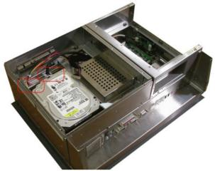
5. Undo the seven screws of the HDD Module so you can install the SDRAM.
